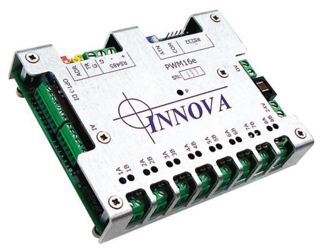
The PWM16 is a member of the Innova Cute family of intervention control products. The unit is a compact, intelligent valve controller with the capability of controlling up to 16 proportional valve functions, as well as pressure sensor monitoring. The unit is designed for mounting in oil-filled compensated enclosures, and pressure rated to 3000msw.
