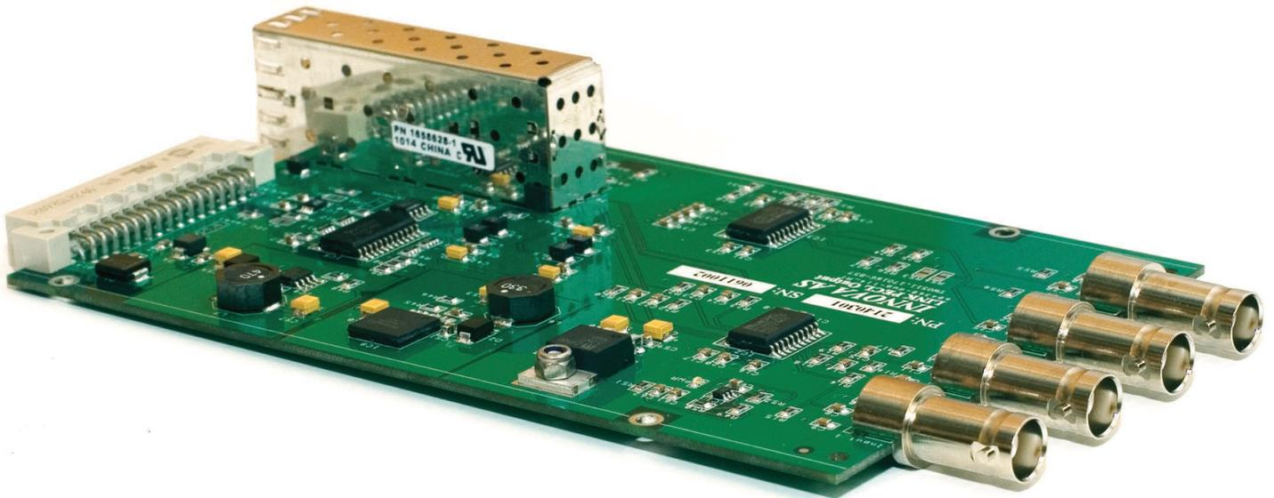
**The Innova Link PECL multibeam sonar interface is a flexible solution for integration of single or dual head multibeam sonars to any remotely operated system.**
