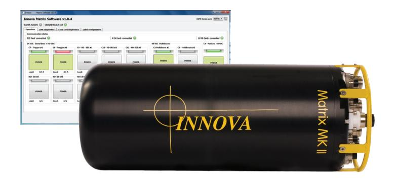
The Matrix is a standalone simple "all in one solution", enabling for transmission of "all you need simultaneous". The system delivers very low-latency, transparent data transmission for a wide range of data formats over a single fibre. The system consists of a compact, one-atmospheric subsea unit rated for 3000 msw, optional 6000msw and a 19" rack mount topside unit. The Matrix enables for conversion of a work class ROV to a survey sensor carrier.
