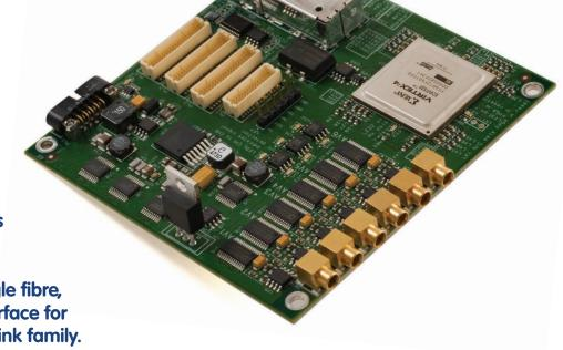
The Innova Link AV video and serial multiplexer is the core system in Innova's fibre optic product family. The system provides video and serial lines over a single fibre, as well as diagnostics interface for the other products in the Link family.
