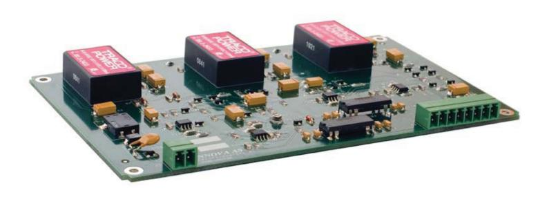
The insulation measurement board will measure the insulation resistance between a low voltage DC (24VDC) powered system and protective earth. Measurement is done by a low current DC signal, in principle as an Ohm-meter. The insulation board can be supplied with 1 or 2 channels for measurement of up to 2 separate (galvanic isolated) powered systems. The output is voltage corresponds to the leakage resistance between the DC powered system and protective earth.
