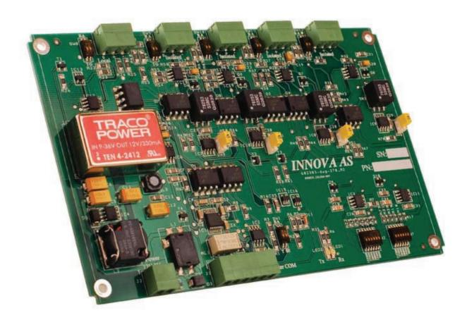
The communication distribution board connects galvanic isolated RS485 networks together and makes them accessible to a master. Communication to master system can be either RS232 or RS485.
