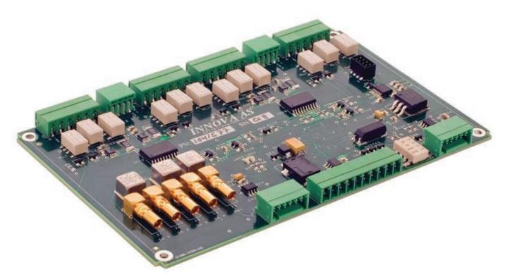
The camera controller board is designed to provide necessary functionality to control 4 cameras and lights used in subsea intervention systems.
