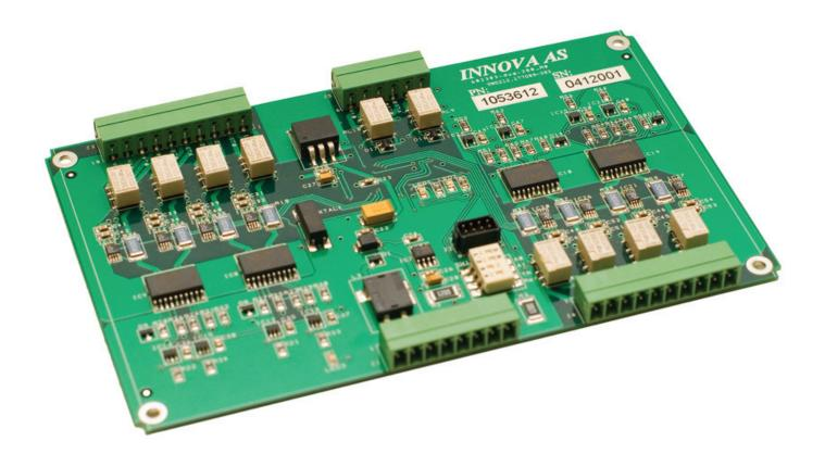
The 10 channel Power Controller board provides power switching to 10 separate power outputs. Communication is by RS232 or RS485.
