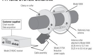
Electronics completion package: Part # 060-G834-03 includes Model 2145 ac receiver, Model 2175A induction power supply, 15 feet coaxial cable, and operating manual.
