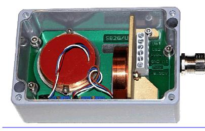
Sensor box containing two NG inclinometers and two signal conditioners with 0...5V outputs and extensive temperature drift compensation
