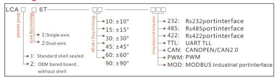
E.g: LCA326T-10-232: Dual-axis/standard/±10°Measuring range/RS232 output
