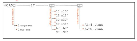
E.g: HCA528T-10-A1: Dual-axis /Standard/±10°Measuring range /4-20mA output current
