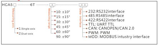
E.g: HCA526T-10-232: Dual axis /Standard/±10° Measuring range/RS232 output
