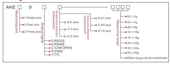
E.g.: AKE192B-02: single-axis、X Axis direction measurement、RS232 signal output、+/-2g selection AKE294B-04: dual-axis、XY Axis directions measurement、RS485 signal output、+/-4g selection AKE39TB-08: three-axis、XYZ Axis directions measurement、TTL signal output、+/-8g selection
