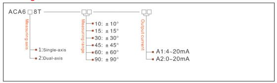
E.g: ACA628T-10-A1: Dual-axis/Standard/±10°Measuring range/4-20mA output current
