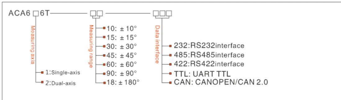
E.g: ACA626T-10-232: Dual-axis/Standard /±10°Measuring range/RS232 output
