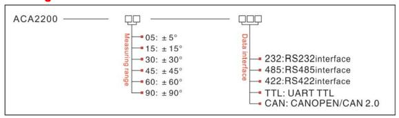
E.g: ACA2200-05-232: Dual-axis/±5°Measuring range/RS232 output
